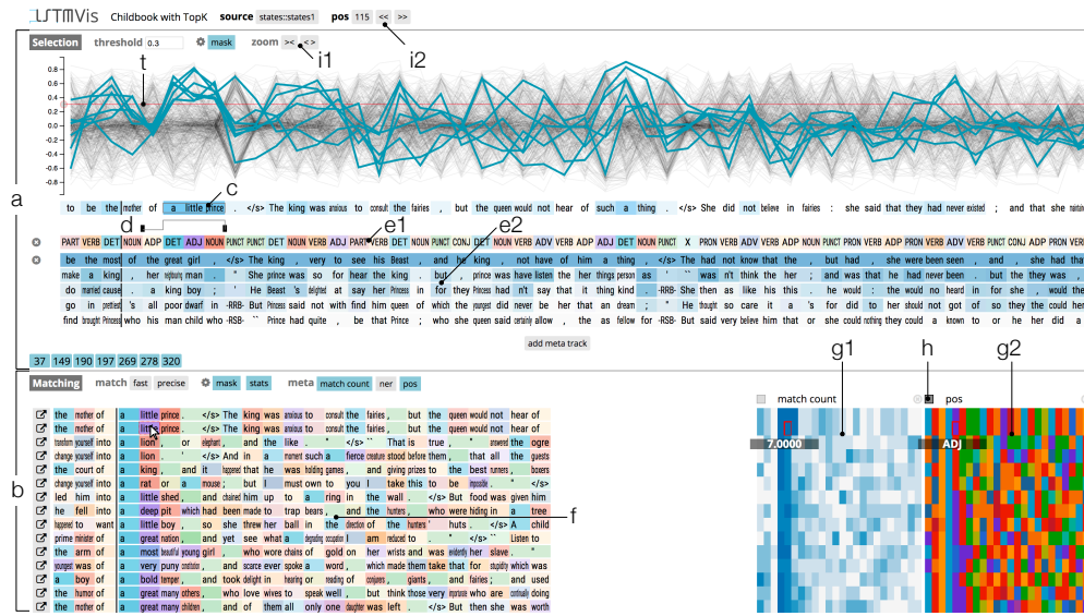
Figure 5.1: The LSTMVis user interface. The user interactively selects a range of text specifying a hypothesis about the model in the Select View (a). This range is then used to match similar hidden state patterns displayed in the Match View (b). The selection is made by specifying a start-stop range in the text (c) and an activation threshold (t) which leads to a selection of hidden states (blue lines). The start-stop range can be further constrained using the pattern plot (d). The meta-tracks below depict extra information per word position like POS (e1) or the top K predictions (e2). The tool can then match this selection with similar hidden state patterns in the dataset of varying lengths (f), providing insight into the representations learned by the model. The match view additionally includes user-defined meta-data encoded as heatmaps (g1,g2). The color of one heatmap (g2) can be mapped (h) to the word matrix (f) which allows the user to see patterns that lead to further refinement of the selection hypothesis. Navigation aids provide convenience (i1, i2).
